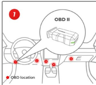
Plug the TopScan into the vehicle's OBD-II port.
