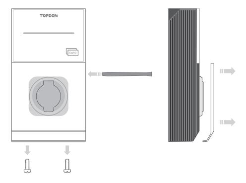
2. Unscrew the eight screws to open the inner cover.
