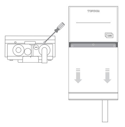
2. Unscrew the eight screws to remove the inner cover.
