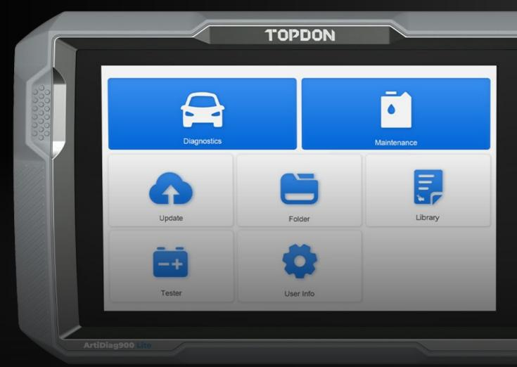
OS: Android 11.0 Storage Capacity: RAM 2G & ROM 32G Screen: 8 inches, 1280\*800 Resolution Connectivity: Bluetooth 5.0/SPP USB Wi-Fi
