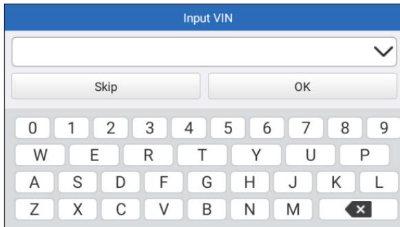
Input the VIN and tap “OK”; the system will automatically identify the vehicle model.
